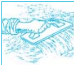
Wood float finish
