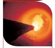
The temperature of the molten minerals in the kiln exceeds 1450°C. Air sucked into the kiln to provide oxygen for the combustion process reaches over 2000°C. These temperatures are necessary for the formation of the clinker.
