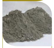
Cement is produced by milling the clinker to a fine powder with the addition of small quantities of gypsum to control the setting time. In producing Cem II cement, unburnt limestone and PFA are also added to reduce the carbon footprint of the cement. The cements are conveyed to silos for dispatch or packed into 25kg bags.
