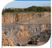
Limestone quarried on-site is the main raw material. Silica and alumina bearing shale, pulverized fuel ash (PFA) from Moneypoint power station and iron ore, are also used. The raw materials are crushed, ground and homogenised to produce a 'raw meal' which is fed to the kiln.
