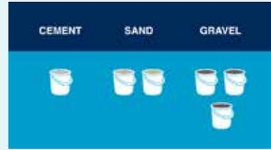
**STEP 2** You can work out the quantities you need by measuring the length by the width by the depth. This applies to all jobs no matter how big or small.
